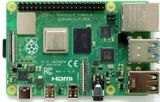
Figure 1. Raspberry Pi 4 circuit parts
